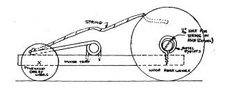
Mount rear wheels on the rear axle. Be sure that the wheels turn freely and do not bind against the body block. Spacers may be needed to aid in this. Front wheels - Remove any molding flash from wheels.
