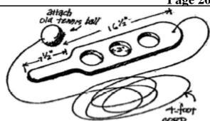
Cut out paddle from  $\frac{3}{8}$ " or  $\frac{1}{2}$ " soft wood. Make 3" holes separated about  $\frac{1}{2}$ " apart. Bevel the handle or sand smooth. Attach an old tennis ball to a strong, four foot cord and tie to the paddle. The object of the game is to toss the ball in the air and catch it in one of the holes.
