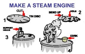
A Webelos Scout may get a graphic demonstration of the power of steam by building the simple steam turbine shown in this illustration. Materials needed are a tin can, a lid from a second tin can, a pair of tin snips, a sheet metal screw, a cork, a power drill, an extra piece of tin to make the support for the turbine wheel, a finishing nail, and a source of heat.
