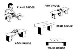
**Beam Bridge:** A beam bridge was derived from the log bridge. It is built from shallow steel beams, box girders and concrete. Highway overpasses, flyovers or walkways are often beam bridges. A horizontal beam supported at its ends comprises the structure of a beam bridge. The construction of a beam bridge is the simplest of all the types of bridges.
