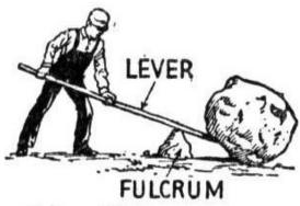
Man lifting a stone with a lever
