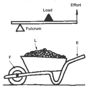
Perhaps the simplest machine of all for increasing force is the lever. A wheelbarrow is a kind of lever and many other types of complicated machines are really just collections of levers that are put together to work in different ways.
