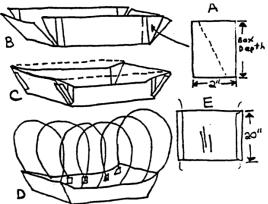
Slit corners open. Cut 2-2" pieces of card- board (box cover) depth of box. Cut each piece in half as in diagram A. Paste one to each corner (B). Tape box Closed.
