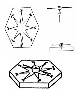
The face of the compass may be cut from  $\frac{1}{4}$ " plywood,  $\frac{1}{2}$ " plywood, or  $\frac{1}{2}$ " pine. The markings for the dial may then be applied with dark crayon, paint, or wood burning.
