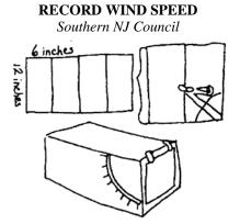
To see how fast or slow the wind blows, make an anemometer (a wind speed measurer)
