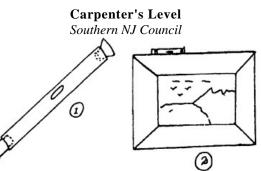
You can make a carpenter's level out of a glass tube - like dentists use or the kind of plastic tube a toothbrush comes in.
