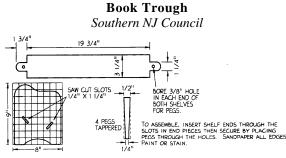
Copy picture and enlarge. Then trace diagram of book ends onto 3/8" board or plywood. Cut shelves from measurements. Make ends identical by clamping together before cutting and finishing.
