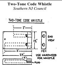
You can work out a series of code signals with this two-tone code whistle. The twin tones make it penetrate a long distance. Each hole may be used independently or both may be blended.
